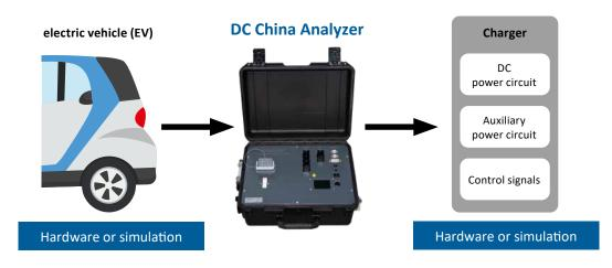
The DC China Analyzer/Simulator supports communication between electric vehicle and charger according to the standards of GB/T 27930-2011 and GB/T 27930-2015, including the support of a simplified SAE J1939-21 CAN transport protocol to handle CAN messages with a DLC up to 512 bytes.
