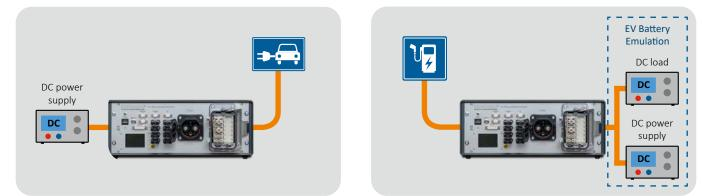
The DC power supply and DC load can be controlled via CAN and have an integrated comemso interface.
